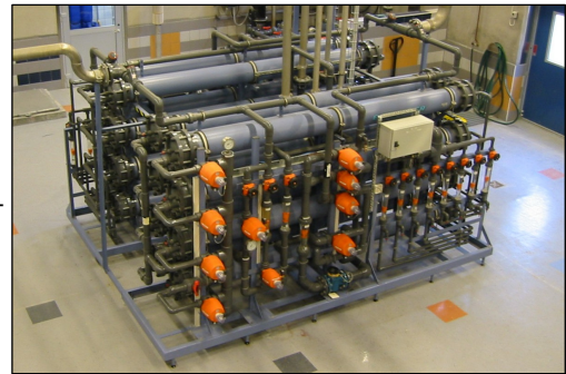
Swedish drinking water plant of 48 m 3 /h. The plant consists of 2 x NF 03-24, prefilter and fully automatic cleaning unit. Application: softening of ground water.
